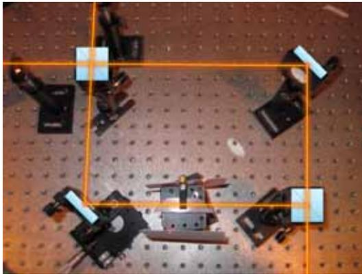
Figure 9: A snapshot of the MZI used in our experiment taken from above. The overlay demonstrates the symbolic representation of the beam splitters and mirrors. The beam splitters are the square boxes with a diagonal slash, and the mirrors are the rectangular boxes. A dove prism can be seen on one arm of the interferometer. Using two dove prisms, we could reproduce the sorting scheme carried out in [9].
