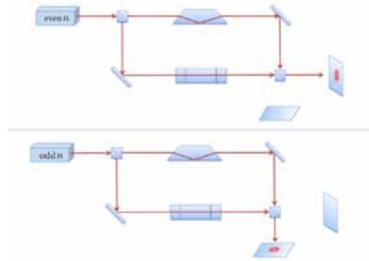
Figure 10: An MZI set up with dove prisms rotated by  $\pi/2$  with respect to each other. The light coming in the MZI is interfered and LG modes with odd and even  $n$  exit the beam splitter perpendicularly provided that each arm has the exact same optical path length.
