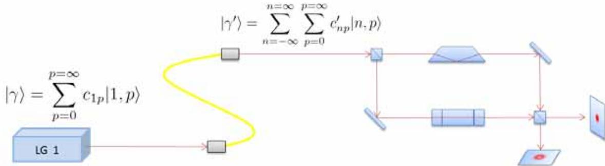
Figure 12: Fiber Distortion. This schematic represents how we can understand the paraxial evolution of the beam in terms of the eigenbasis we have constructed in (12). A prepared LG 1 mode is coupled to a fiber optic channel. The fiber distorts the output beam which can be seen as a transformation  $|\gamma'\rangle = F|\gamma\rangle$ .
