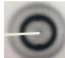
Example of a diffraction pattern
