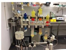
BioRad purification system with column
