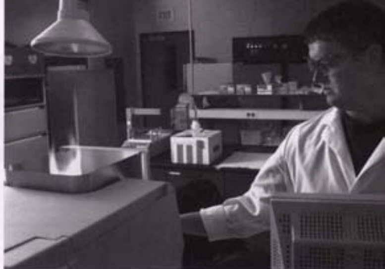
Graduate student Royce Hughes analyzes water samples for heavy metals using an atomic absorption spectrometer.
