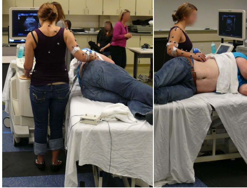
Figure 4: Reflective markers and surface electromyography electrodes on a sonographer participant while she is scanning the right kidney of the patient
