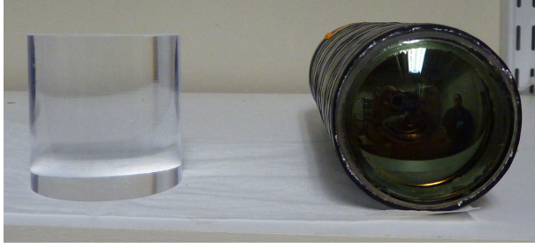
Figure 10: Fast plastic scintillator cylinder and photomultiplier tube.
