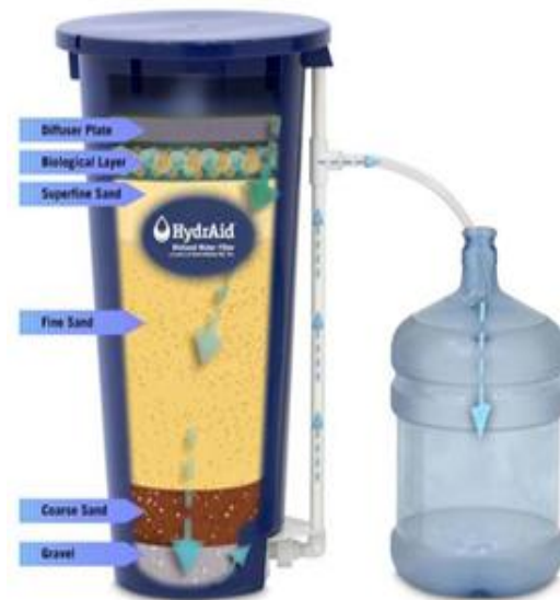
Figure 1.1. Profile view of the HydrAid® Biosand Filter manufactured by Cascade Engineering, Grand Rapids, Mi.
