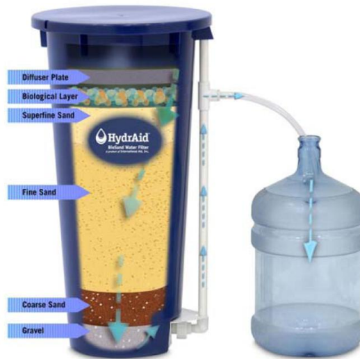
Figure 4.1. Profile view of the HydrAid® Biosand Filter manufactured by Cascade Engineering, Grand Rapids, Mi. Picture adapted from HydrAid® Manual.
