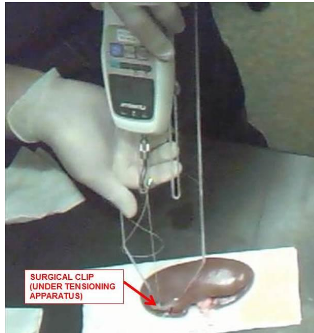
Figure 7: Handheld Tension Measurement
