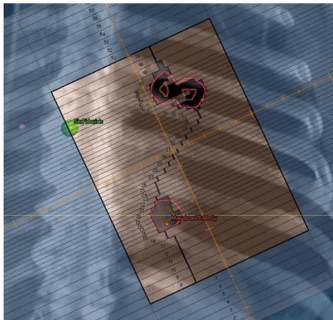
Figure 1. Display of isocenter placement and collimator selection
