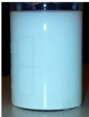
Figure 10: TiO 2 suspension two weeks after preparation that began with 20 \mu m TiO 2 particles and incorporated both ethanol and PEG20000. Preparation included 2 hours of milling.
