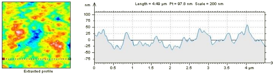
Figure 16: Profile line nearer to the perimeter of the same TiO 2 surface area as Figures 16 and 17. A higher degree of surface variation existed in this region of the scan.
