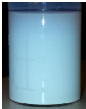
Figure 7: Two week old nanoparticle \text{TiO}_2 suspension, pH adjusted DI water, and PEG600 equal to at 50% the weight of the \text{TiO}_2 . Dispersion in the main volume of the suspension was maintained.
