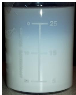
Figure 8: Two week old suspension with 20% Ethanol by vol., 2% TiO 2 by wt., and pH adjusted DI water as the primary solvent. Sediment layer on the bottom of the beaker was observed to be less than 1% of total volume.
