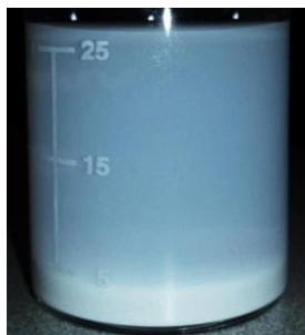
Figure 5: Two week old suspension with no PEG component. A relatively thick sediment layer formed on the bottom of the storage beaker indicating poor stability. The height of the sediment observed in the sample was measured to be 15% of the total height of the suspension.
