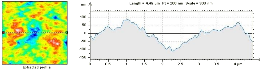
Figure 15: Profile line cutting through pore in the center of the scanned area the previous figure.
