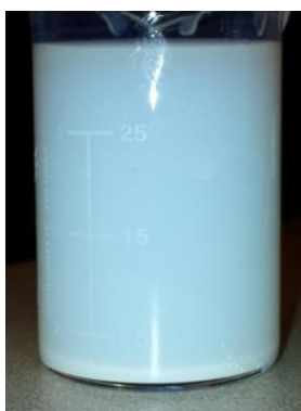
Figure 9: Two week old sample with an 80% ethanol content. The bottom sediment layer is thicker than the 20% content, indicating an acceleration of sedimentation. The upper region shows a nearly uniform distribution.
