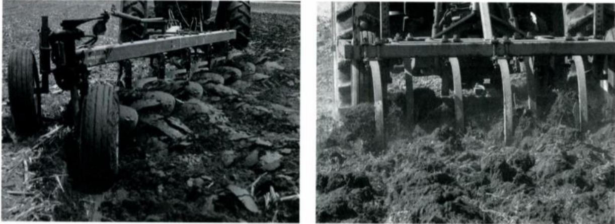
Figure 2. (Left) In conventional tillage, a moldboard plow inverts the upper soil horizon, burying all plant residues and producing a bare soil surface. (Right) A chisel plow, one type of conservation tillage implement, stirs the soil but leaves a good deal of the crop residues on the soil surface (Brady & Well, 2008, p. 763; Photos courtesy of R. Weil).
