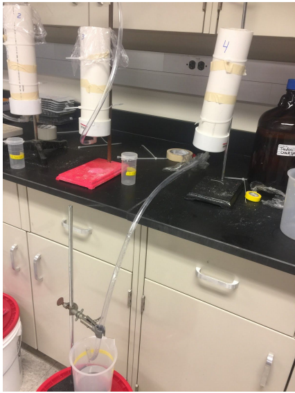
Figure 2. Setup of the filter with hose leading to collecting vessel.
