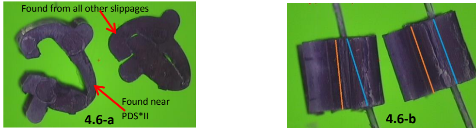
Figure 4.6. Open LAPRA-TY® recovered from tank, 4.5-a, and inconsistent clipping of LAPRA-TY® on a PDO size 3-0 sample, 4.5-b (the photos were taken at 28 times magnification using Brown & Sharpe Coordinate Measuring Machine; courtesy: Medbio, Inc.)
