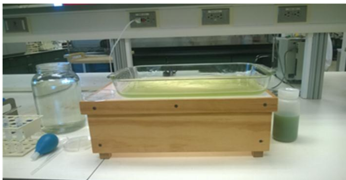
Figure 3.1: Counting dish above a lightbox, used for sediment evaluation and colony counting.
