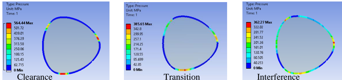
Figure D20: Contact stress in the P3G shaft along the edge for torsional load
