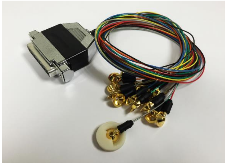
Figure 3-5. The 16 gold cup electrodes with 25-pin D-sub connector to the wireless acquisition unit. The prototype version of the electrode adapter is also shown.
