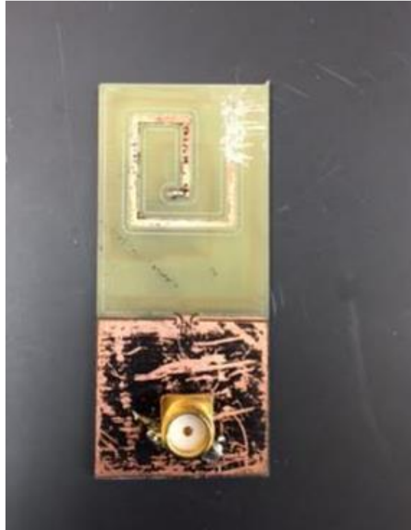
Figure-4.3: Antenna prototype tuned to resonate in MICS band.
