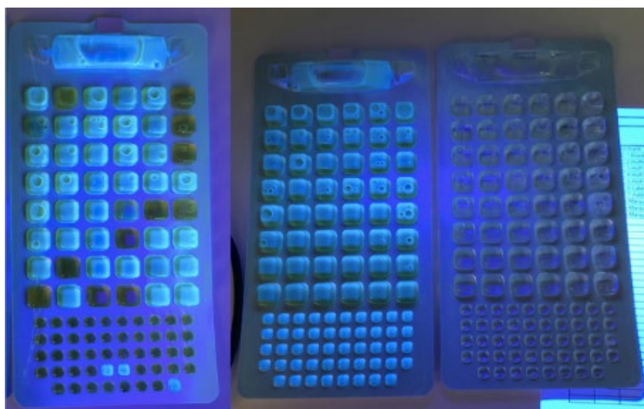
Figure 6. Example of Colilert-19 Sample Trays with Many Fluorescent Wells (Left) and All Wells Fluorescent (Center) and One Blank Tray with No Fluorescent Wells (Right).
