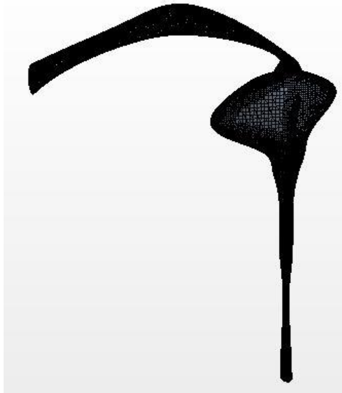
Figure 15. Volume mesh of poor VPRM case (5.9 Million cells)
