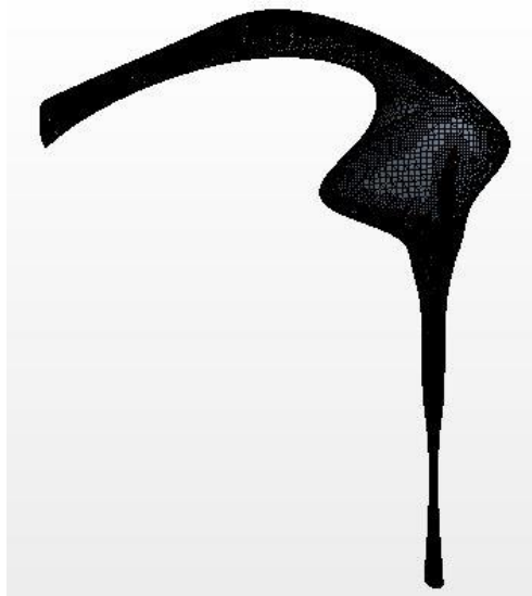
Figure 13. Volume mesh of Regular case (6.45 Million cells)
