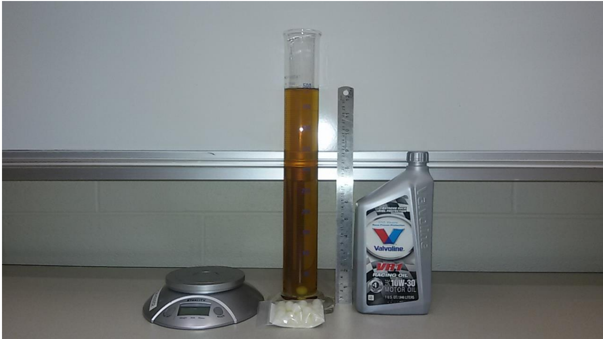
Figure 2. Experimental setup for Stokes falling sphere experiment
