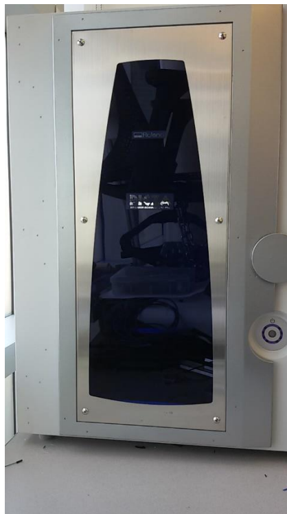
Figure 4. Roland LPX600 3D scanner
