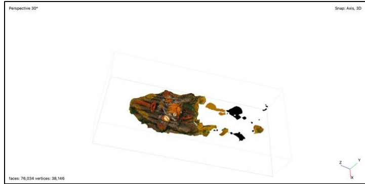
Figure 18: Movement of the cord results in multiple cords appearing in the model. Similarly, to the belt, attempting to fix this issue results in the removal of the cord altogether. This issue can only be corrected by repeating the photo process.
