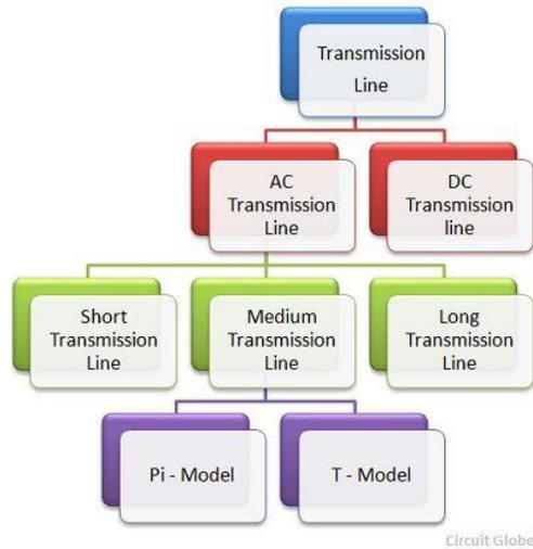
*Figure 2: Classification of Electrical Transmission Line [Courtesy Circuit Globe]*
