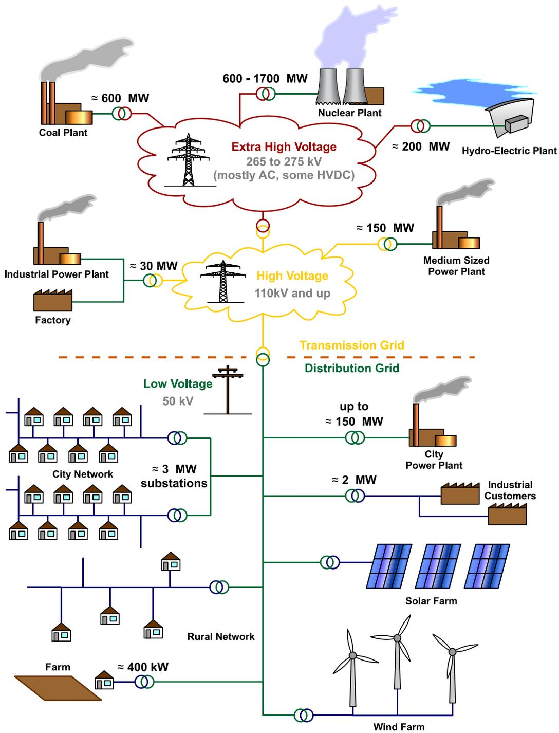
Figure 3: General Layout of Electricity Network [Courtesy <https://commons.wikimedia.org/w/index.php?curid=9676556>]
