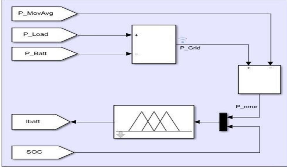
Figure 38: Inside view of Fuzzy controller block
