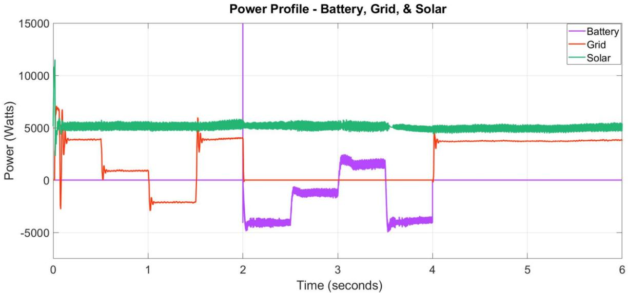
Figure 43: Power Profile of step 1 simulation showing Battery, Grid, and Solar Power
