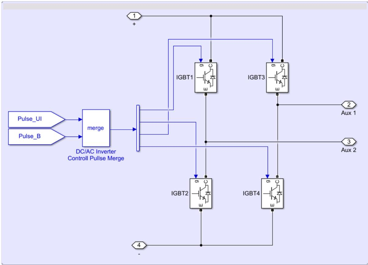
Figure 41: IGBT based DC-AC Inverter model
