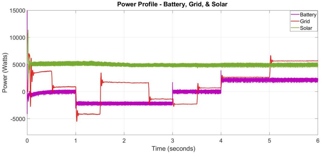
Figure 49: Power profile of step 2 simulation showing battery, grid, and Solar
