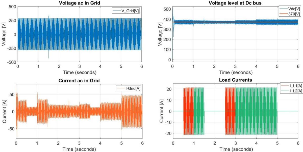
Figure 48: Voltage and Current at House 1 and Vdc maintained at 370V in step 2
