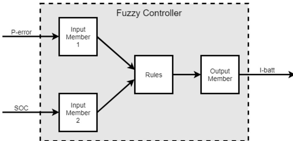
*Figure 29: Fuzzy Controller Block Diagram*
