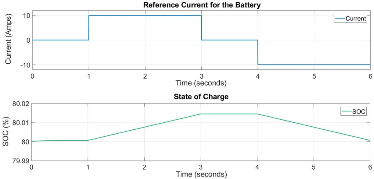
Figure 47: Reference Current for the battery and the State of charge SOC of the battery
