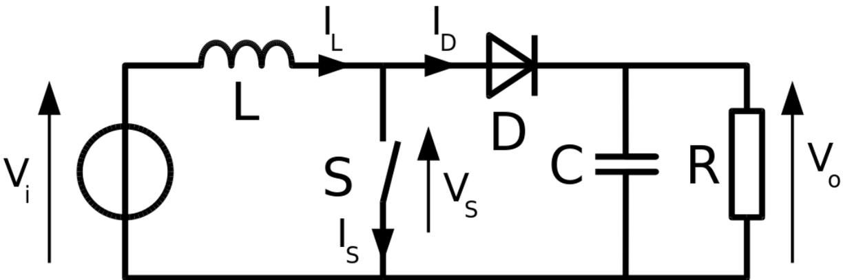
Figure 13: Boost Converter Circuit
