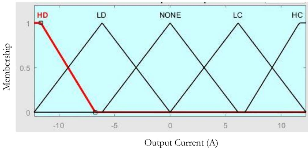
Figure 33: Output Membership Function plot – I-Batt (shown for small battery)
