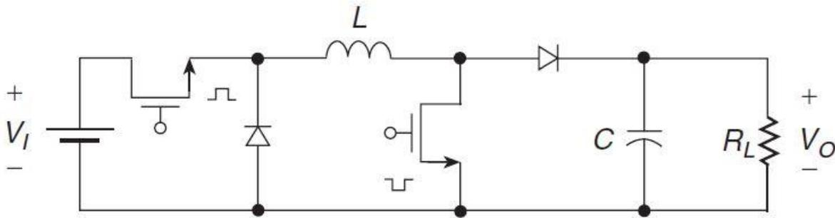
Figure 14: Non-inverting two switch buck-boost converter [42]
