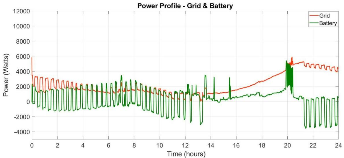
*Figure 55: Step 3 simulation – grid and battery power profile for medium battery on day 1*
