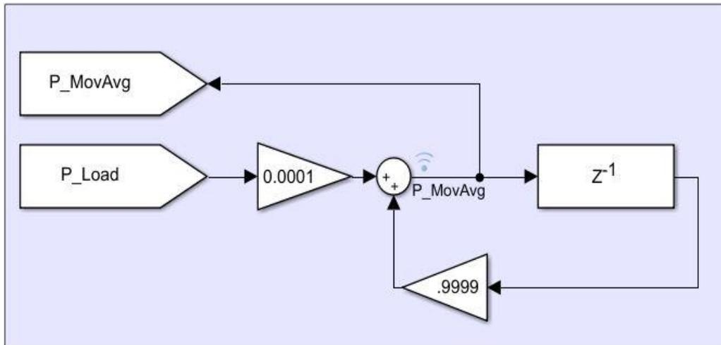
Figure 36: Inside view of moving average calculation block
