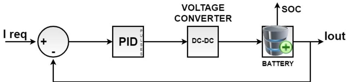
Figure 27: Control Scheme for Battery Current
