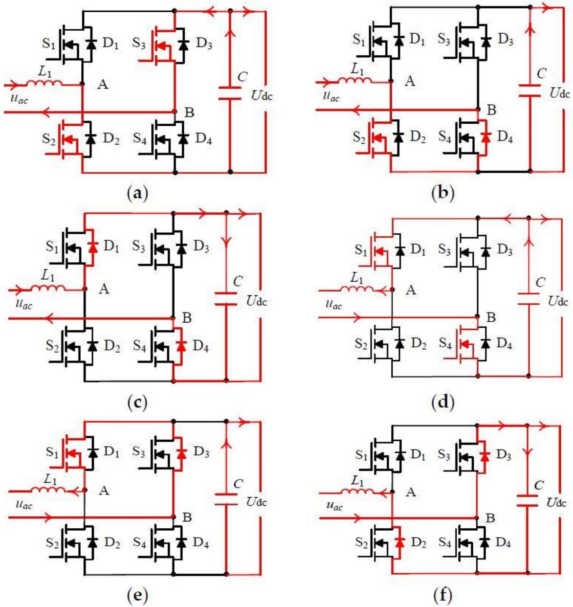
Figure 18: AC-DC battery charging mode [44]
