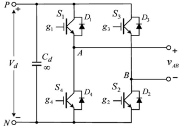
Figure 15: Single phase H-bridge Inverter [43]
