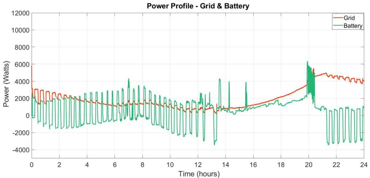
*Figure 59: Step 3 simulation – grid and battery power profile for big battery on day 1*
