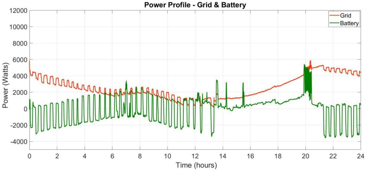
*Figure 57: Step 3 simulation – grid and battery power profile for medium battery on day 2*
