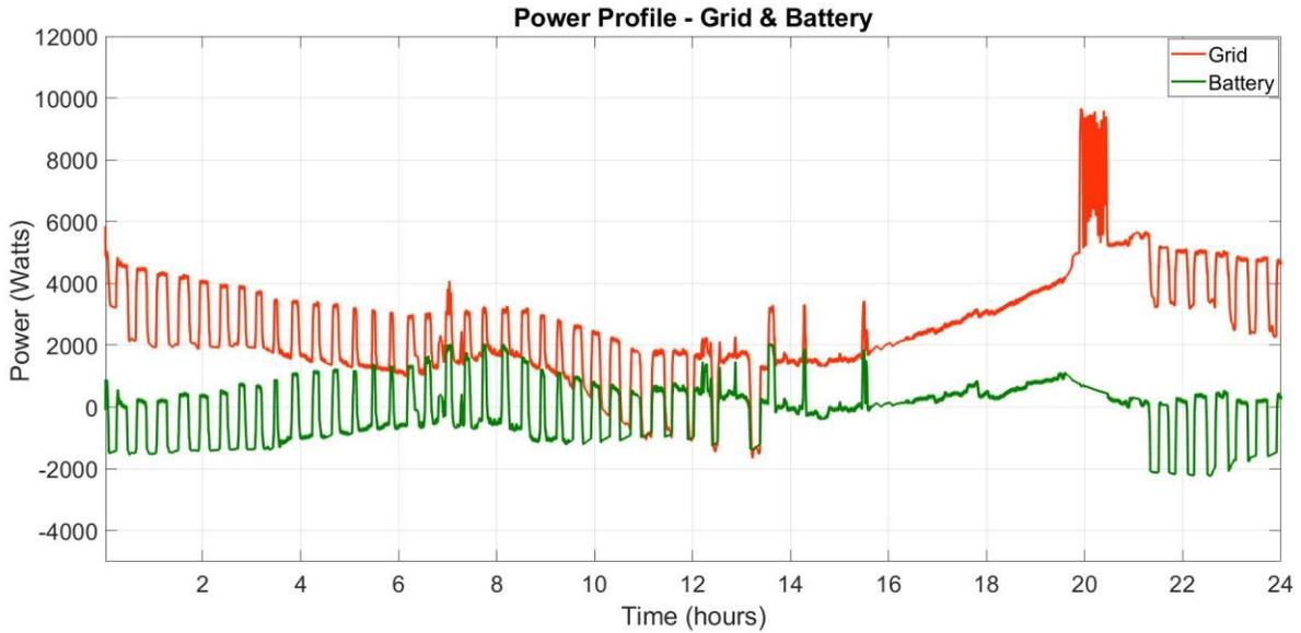
Figure 53: Step 3 simulation – grid and battery power profile for small battery on day 3
