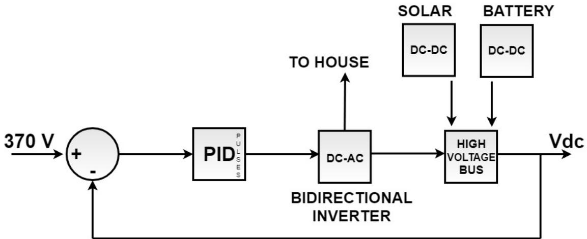
Figure 26: Control Scheme to maintain voltage level
