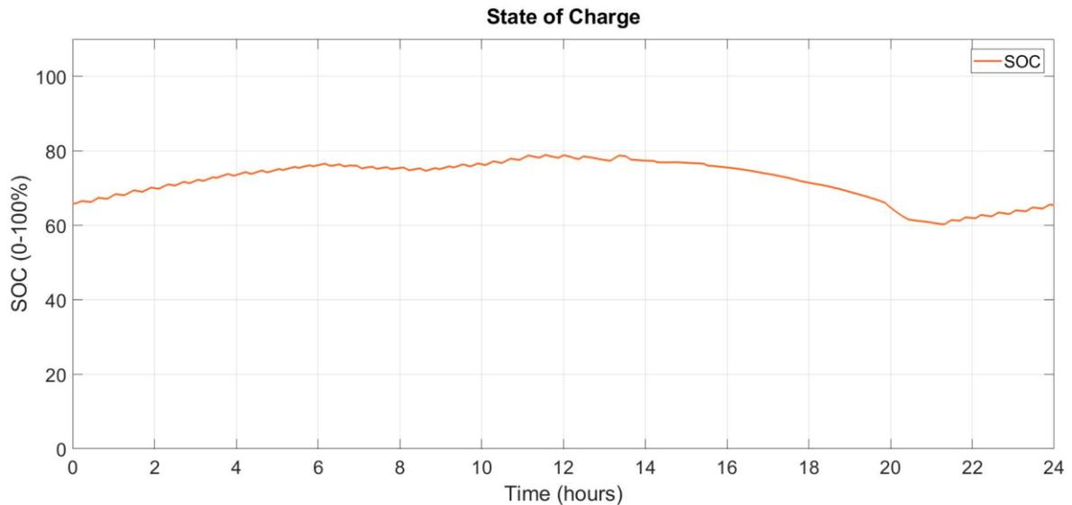
Figure 62: Step 3 simulation - State of charge of the big battery on day 2
