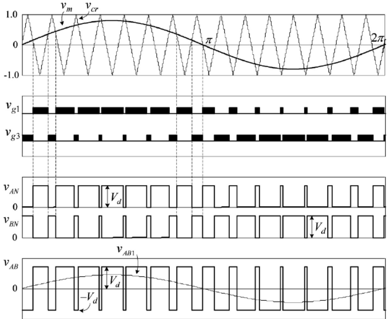
Figure 16: Waveform of Bipolar modulation [43]
