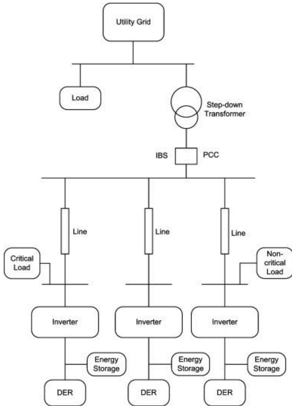
Figure 11: Application of Inverter and energy storage in storage in grid [34]
