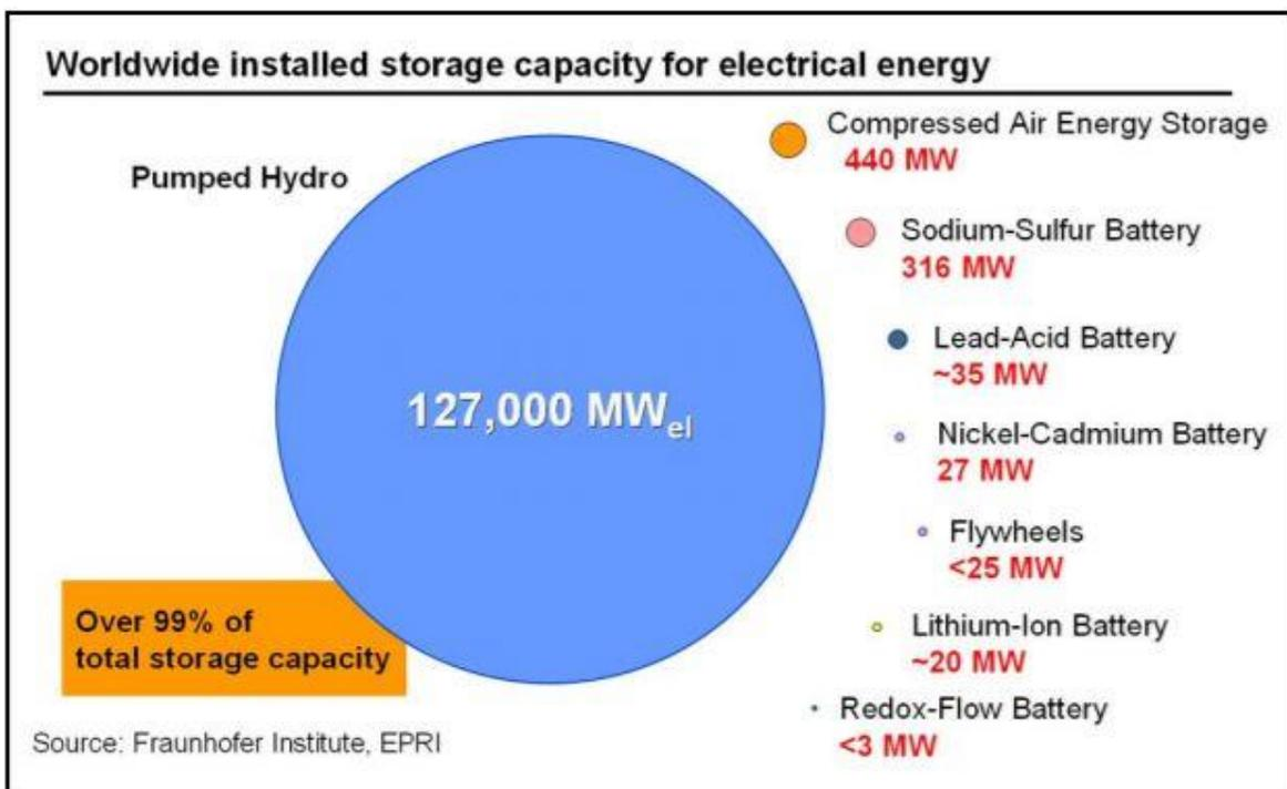
Figure 8: Worldwide installed storage capacity for electrical energy [40]
