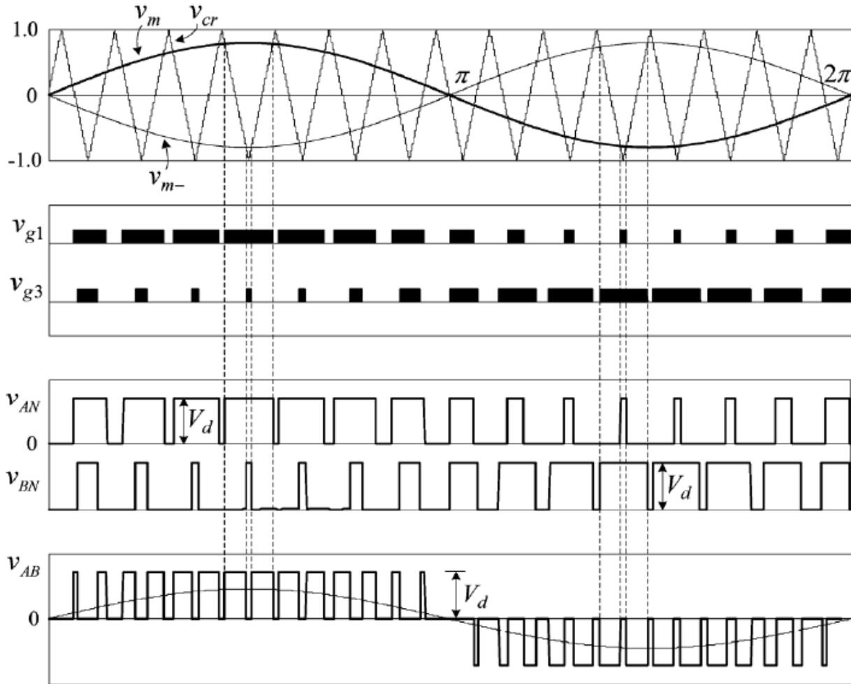
Figure 17: Waveform of Unipolar Modulation [43]
