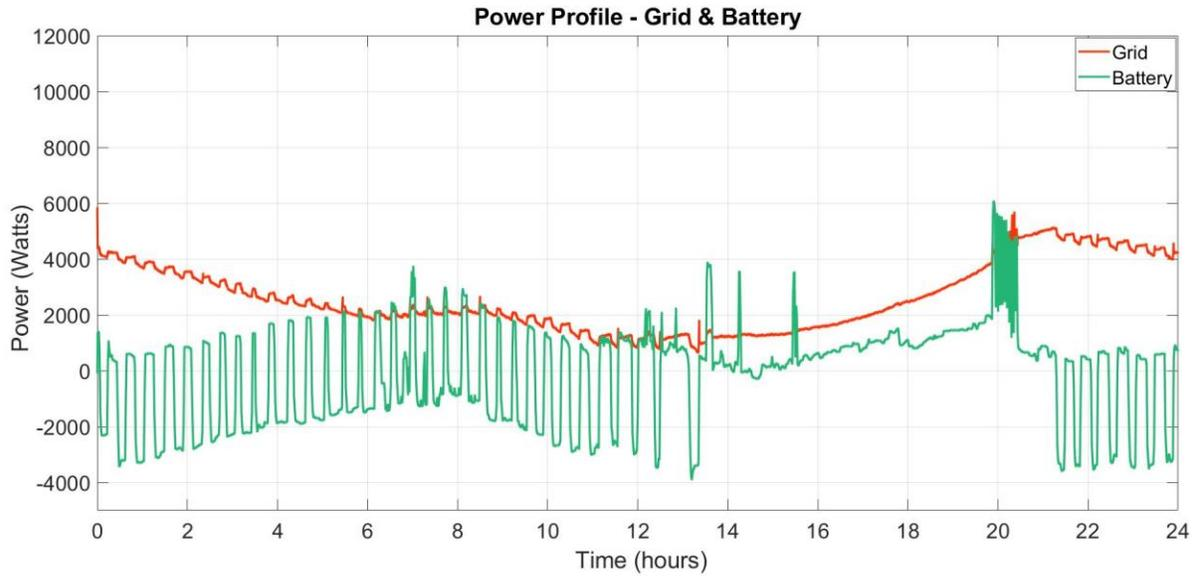
Figure 61: Step 3 simulation – grid and battery power profile for big battery on day 2
