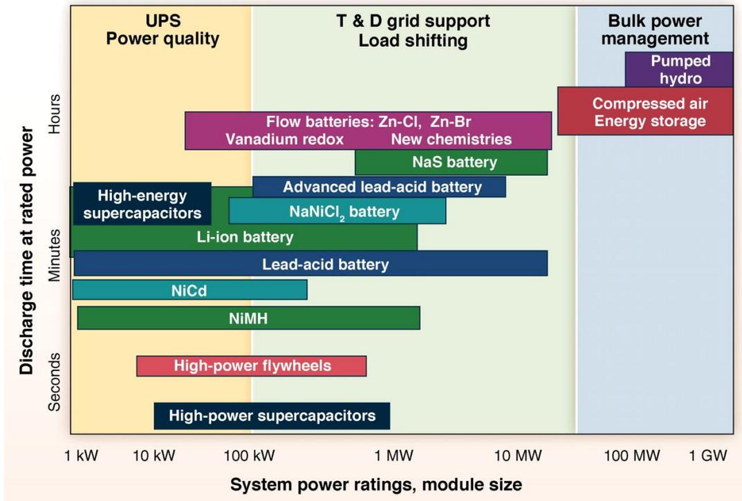
Figure 9: Comparison of discharge time and power rating for various EES technologies [6] [Courtesy of EPRI]
