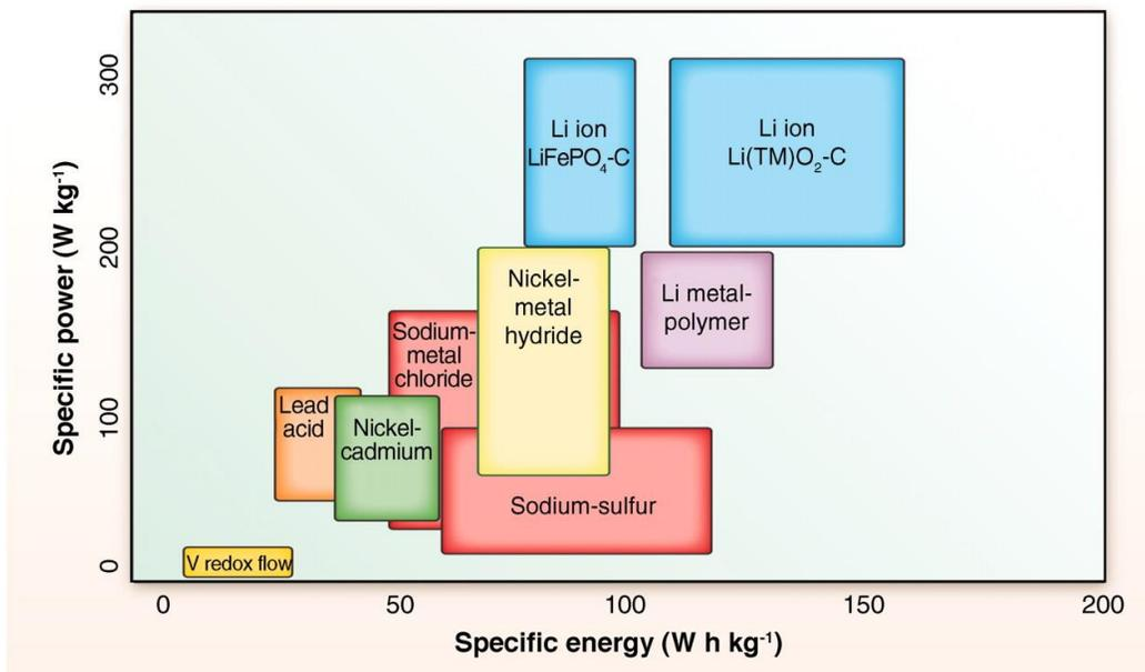
Figure 10: Specific Power vs. Specific Energy of different battery types for EES [32]
