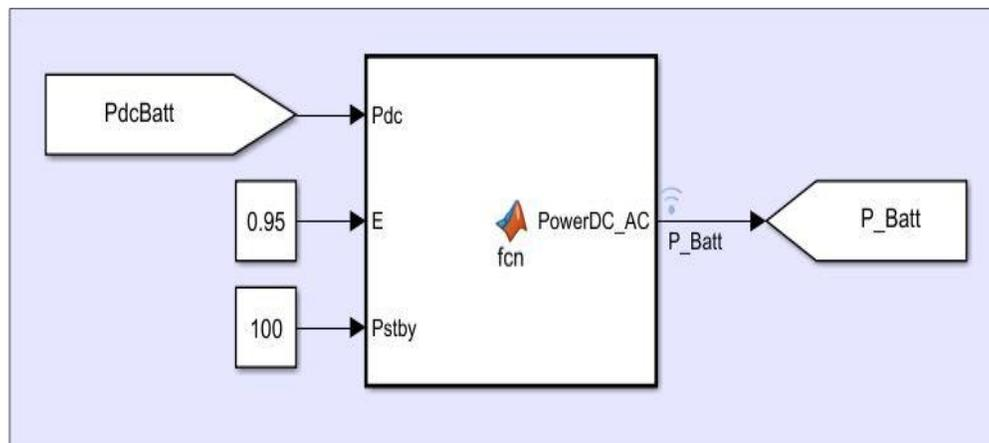
Figure 37: Inside view of power loss calculation block
