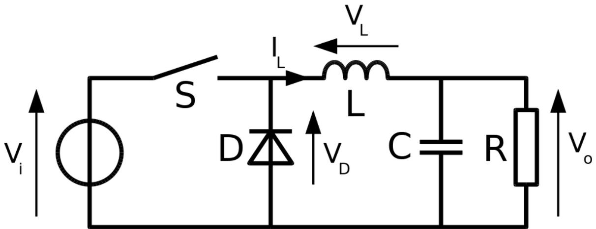
*Figure 12: Buck Converter Circuit*
