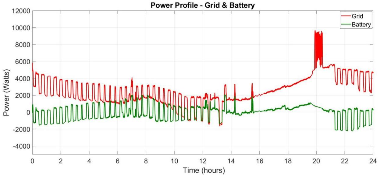
*Figure 51: Step 3 simulation – grid and battery power profile for small battery on day 2*
