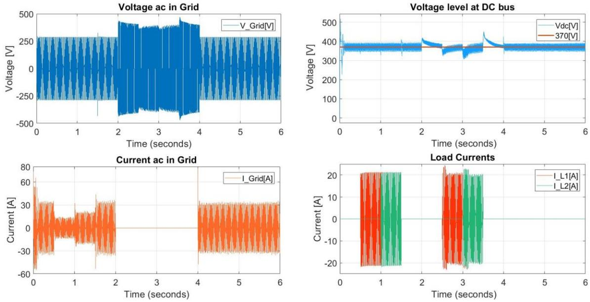
Figure 44: Voltage and Current at House 1 and  $V_{dc}$  maintained at 370V in step 1
