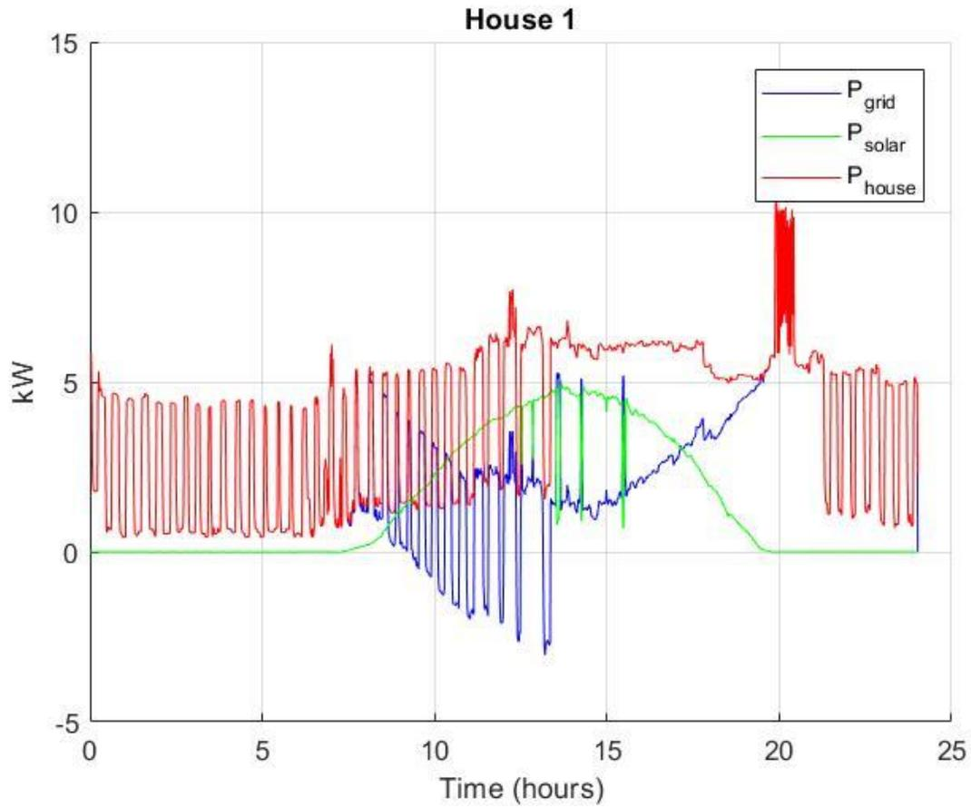
Figure 28: shows house 1 data from Pecan Street Project for a whole day. The data provides Solar power generated, Electricity consumed in the day, and the contribution of power form the electric grid.
