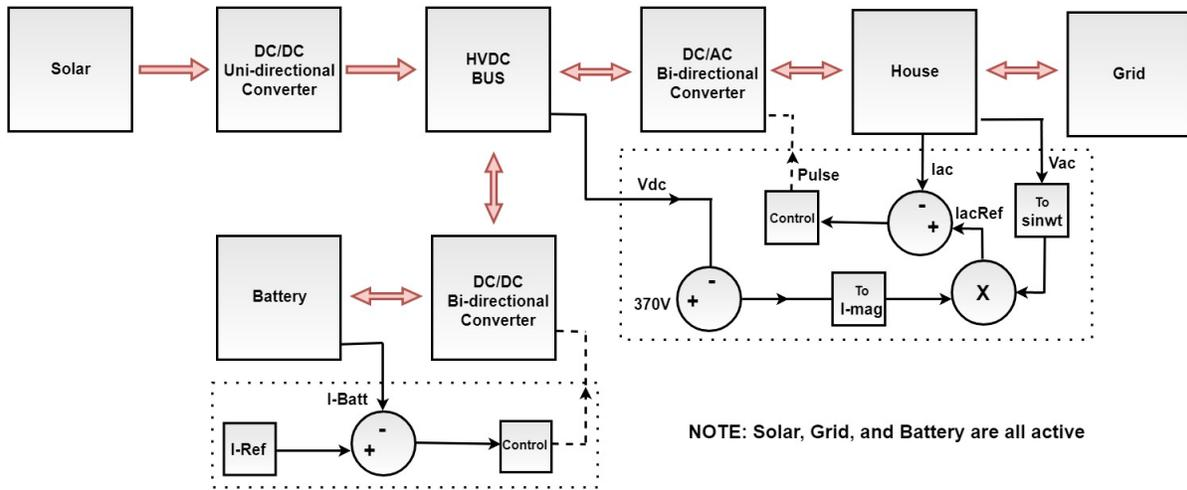
Figure 25: Control loops in step 2 model
