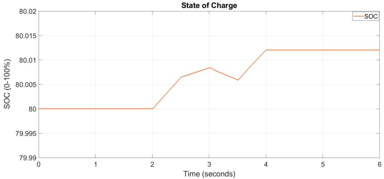
Figure 45: State of Charge SOC of the battery in step 1 simulation
