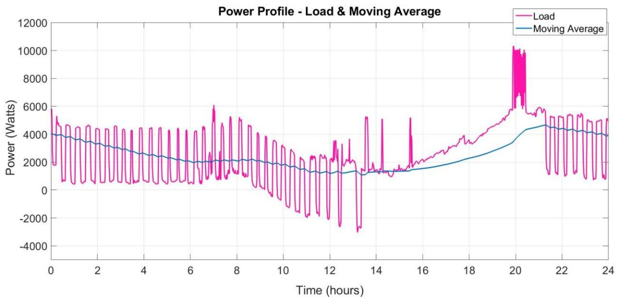
Figure 50: Step 3 simulation power profile - Load and moving average of load
