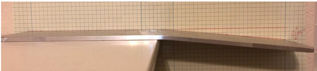
Figure 66: Drop test deformation to aluminum plate with PORON pad.
