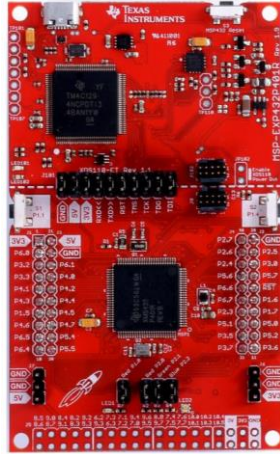
Figure 1: MSP432 Launchpad Diagram[6]
