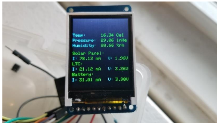
Figure 33: Display showing the ADC result values and BME sensor
