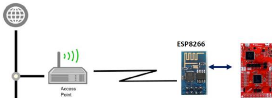
Figure 3: Communication path between MSP432 to the Internet via ESP8266
