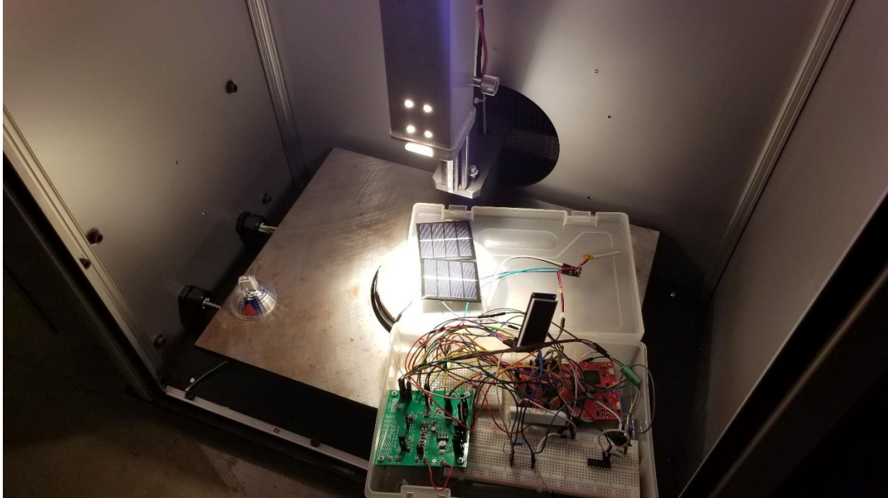
Figure 39: Test setup inside an ELH halogen light box
