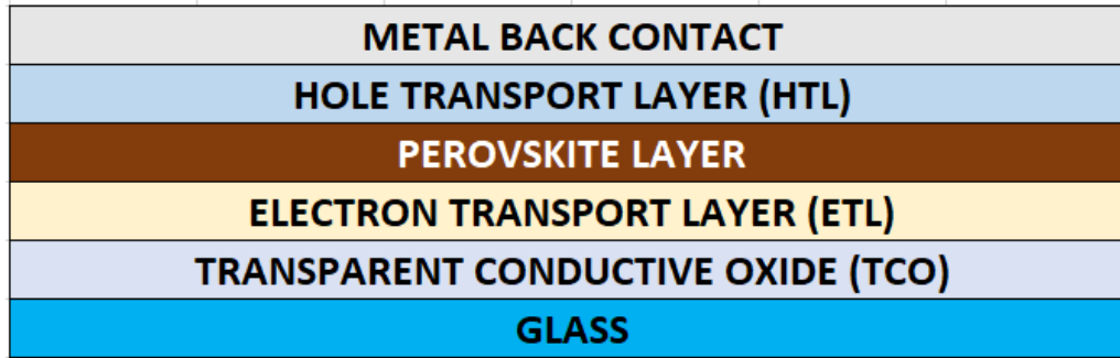
Figure 2: Basic Perovskite Solar Cell Structure
