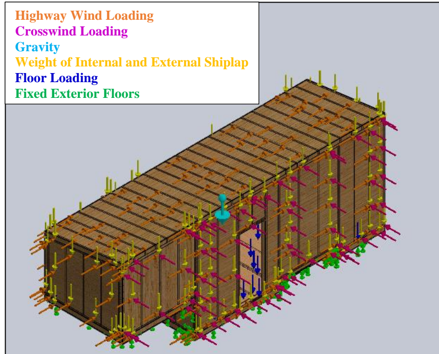
Figure 52: Visual Example of Mobile Boundary Conditions on the Tiny House (Isometric View)
