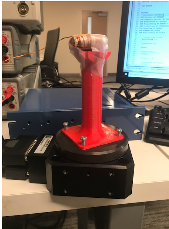
Figure 17: Sensor Mounted to Angular Displacement Control Motor
