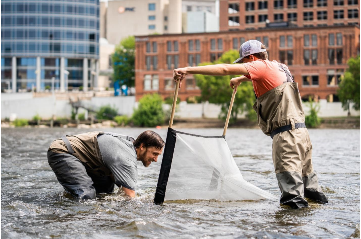
Figure 3. Stanford-Hauer kicknet in operation in the Impact reach of the Grand River, Grand Rapids, MI. 0.5 m 2 of benthos was sampled: first, medium to large substrate was sampled with gloved hands and set aside; next, immovable substrate was hand-scrubbed; and, finally, remaining substrate was kick-sampled for approximately 30 seconds.
