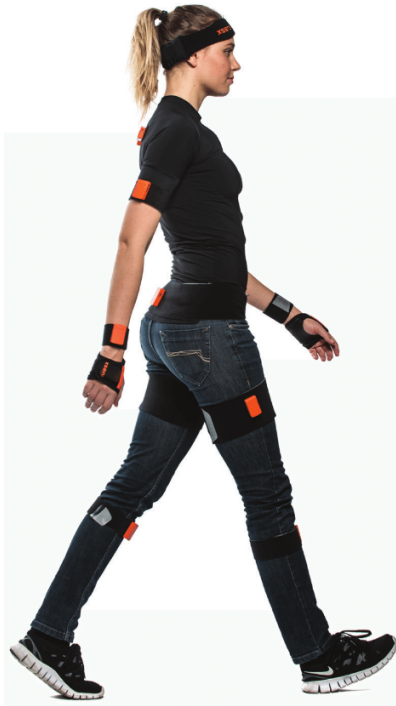
Figure 2. Example of typical XSENS setup with IMU sensors shown in orange [22]
