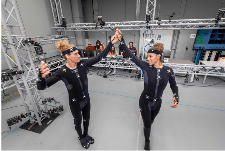
Figure 1. Example of Vicon system with reflective markers on subjects as well as camera and laboratory set up [21]
