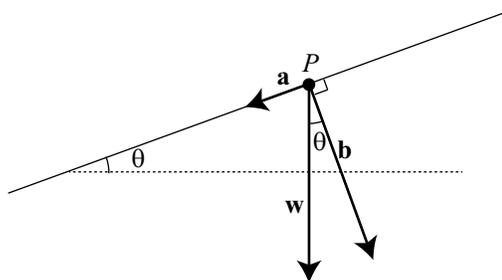
Figure 3.22: Inclined Plane
