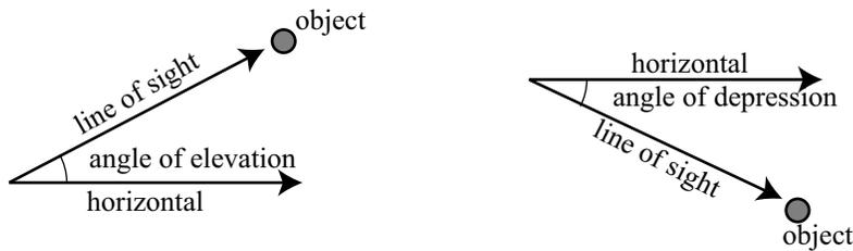
Figure 3.11: Angle of Elevation and Angle of Depression
